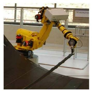
materials which are inserted between the stringers. And also the next step should be automated: the application of a film, which covers the stringers and auxiliary materials.
